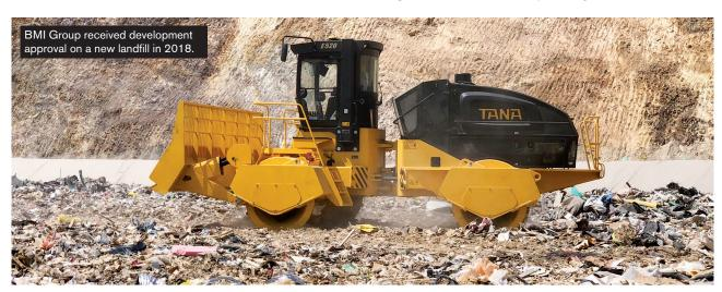
at operator level, while a bigger cab offers 360-degree views in addition to a window from roof to bottom floor for better visibility.
